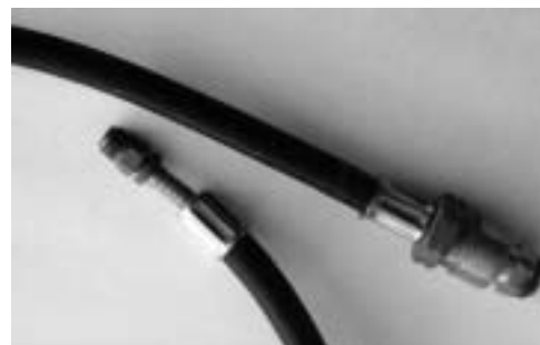
The old hose with the brass fitting separated
