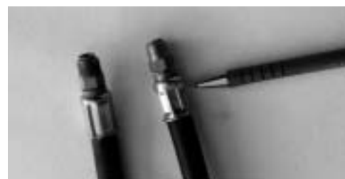
The new hose assembly (indicated by the biro) can be identified by the slightly shorter crimping
