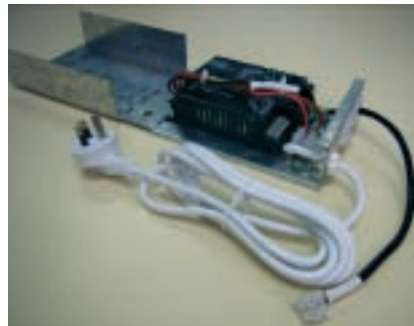
The digital dimmable ballast showing the 2-core switching cable
